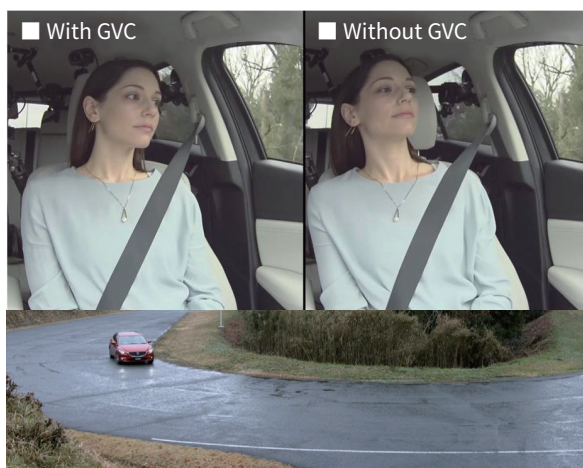
Fig 10 : Reduction in torso-sway with GVC
